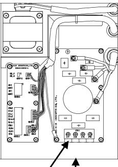
Power supply connection terminal block
