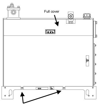
Cross-recessed truss head machine screws
