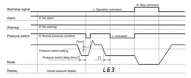
The above chart shows the case where "P08" (Pressure switch display hold setting) is [1] or [2].
