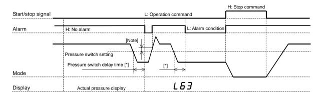
The above chart shows the case where "P08" (Pressure switch display hold setting) is [1] or [2].
