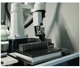
The CPX machine is offered with ANCA's own AR300 low cost loader for automated loading of tool blanks.
