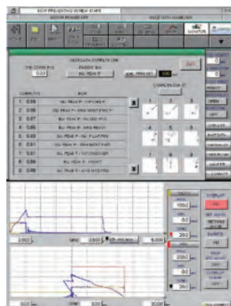
▲Correlation check/injection pressure monitoring
